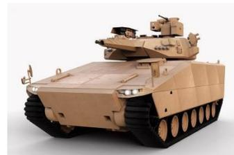
The AS21 Redback is designed to improve the survivability against higher threat levels. It can accommodate eight troops and has a crew of three. The vehicle can be fitted with new generation of APS (Active Protection System) designed to prevent line-of-sight guided anti-tank missiles and projectiles from destroying the vehicle
